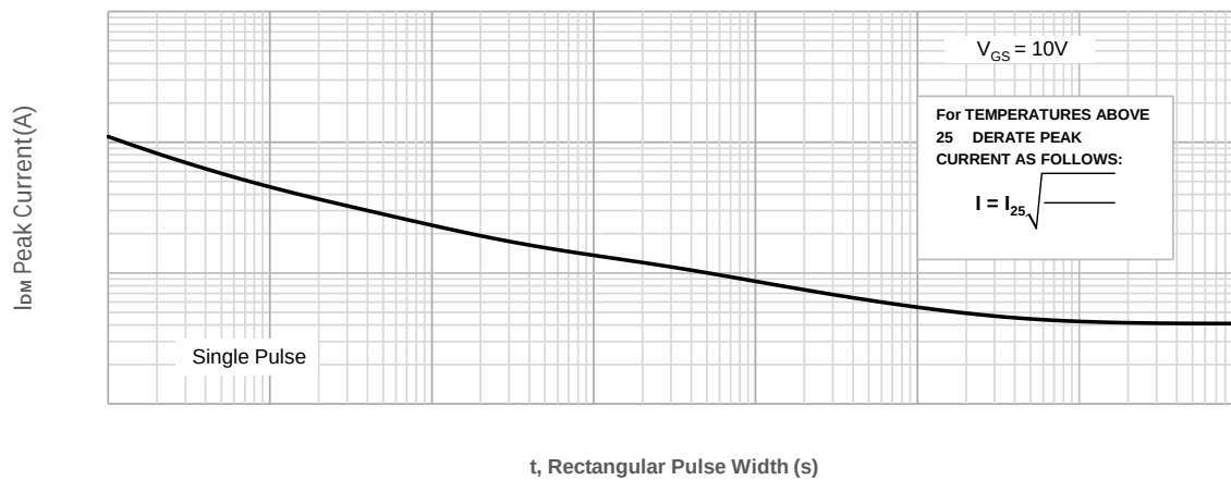
Figure 4: Peak Current Capacity
